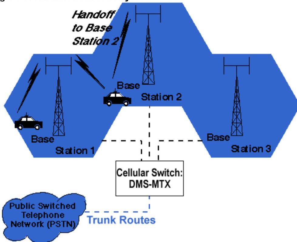
During a call, two parties are on one voice channel. When the mobile unit moves out of the coverage area of a given cell site, the reception becomes weak. At this point, the cell site in use requests a handoff. The system switches the call to a stronger-frequency channel in a new site without interrupting the call or alerting the user. The call continues as long as the user is talking, and the user does not notice the handoff at all.
