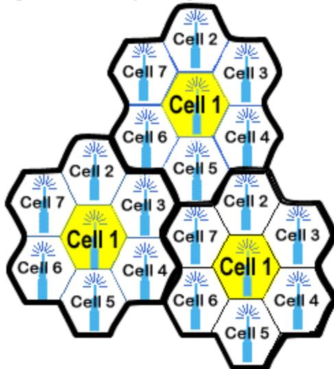
Cells with the same number have the same set of frequencies. Here, because the number of available frequencies is 7, the frequency reuse factor is  $1/7$ . That is, each cell is using  $1/7$  of available cellular channels.
