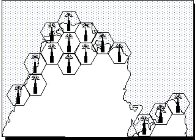
The cellular radio equipment (base station) can communicate with mobiles as long as they are within range. Radio energy dissipates over distance, so the mobiles must be within the operating range of the base station. Like the early mobile radio system, the base station communicates with mobiles via a channel. The channel is made of two frequencies, one for transmitting to the base station and one to receive information from the base station.
